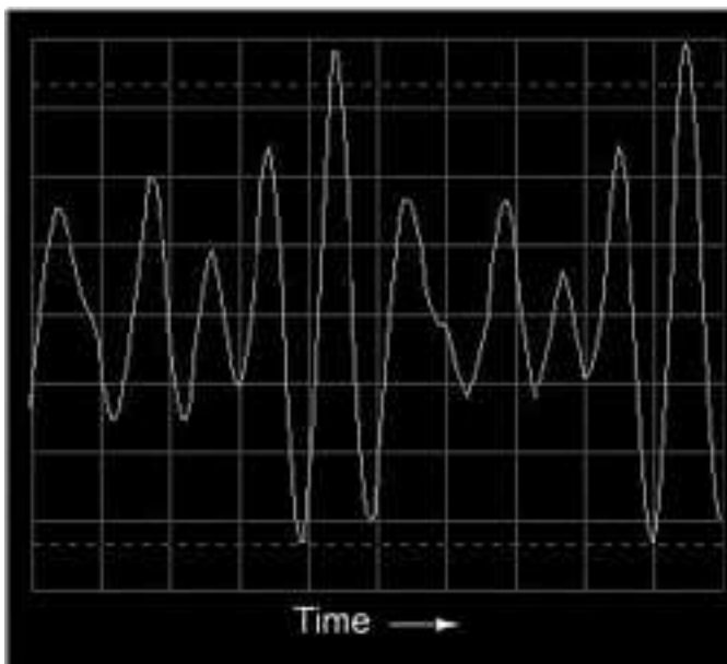
Figure 7.25: Oscilloscope display: three tones.
