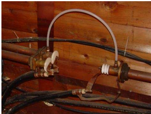
Figure 14.52: Flexible coaxial cables connected to rigid lines.
