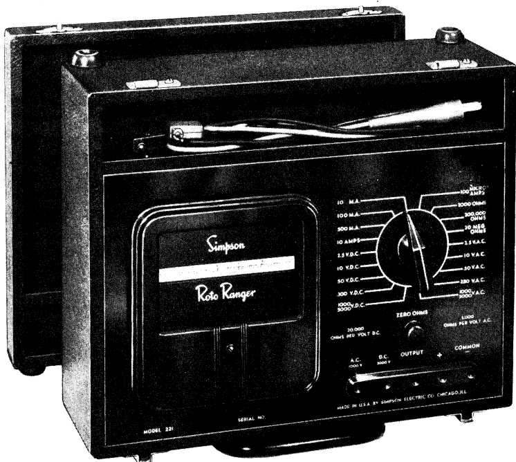
Figure 1 Simpson Model 221 Volt-Ohm-Milliammeter Size: 12 3/4" x 10 1/8" x 5 3/8". Weight 8 lbs. 9 oz.
