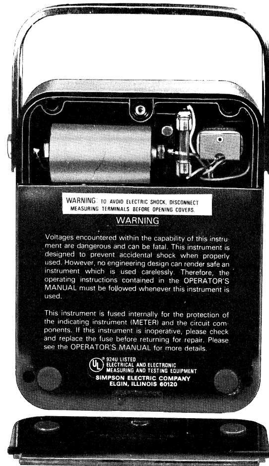
Figure 5-1. Battery and Fuse Compartment.
