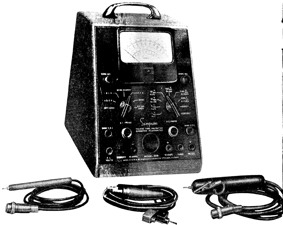
Figure 1 Simpson Model 266 Vacuum Tube Voltmeter Size: 8½" x 9½" x 8". Weight: 8 lbs.
