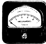
MODELS 127, 137, 147, 157, 2½" RECTANGULAR ACCURACY: 2% SCALE LENGTH: 1-7/8"
